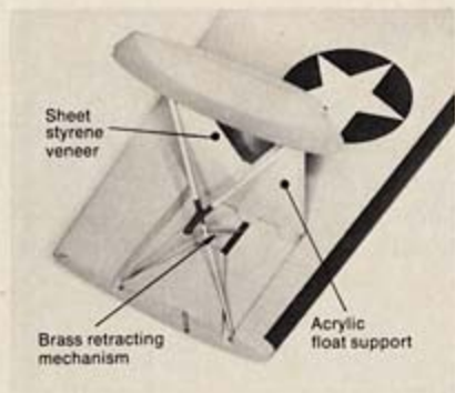
Fig. 18. The Catalina's retractable wing-tip floats were made from acrylic stock, sheet styrene, and brass.
