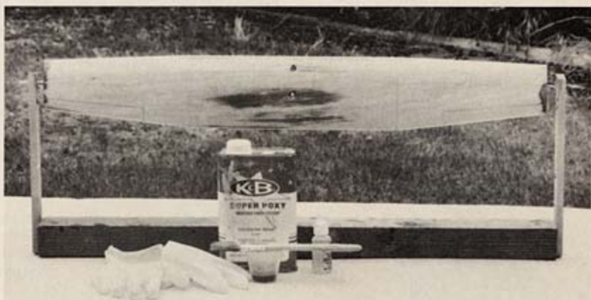
Fig. 13. To hold the wing while applying polyester resin, Paul assembled this rig. Polyester resin has quite an odor, so work outside.
