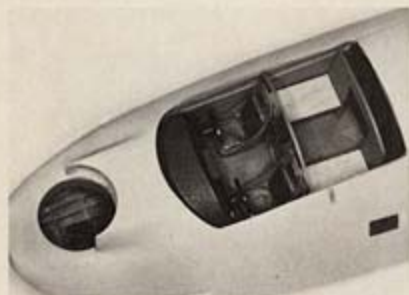
Fig. 8. Both the nose compartment and the cockpit interiors were slipped into the fuselage through the cockpit opening.
